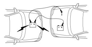
4. Make the final connection of the negative (-) cable to an exposed metal part of the stalled vehicle's engine, away from the battery and the carburetor/fuel injection system.
